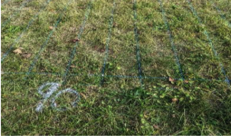
Figure 10: Gridding is a process of marking off the entire area to be scanned with string/twine. To ensure data collection accuracy, grid lines are secured to the ground with large nails at set intervals. Grid lines are fastened to the front lawn area in preparation for the GPR scan; 0.25 meter intervals are used to ensure a high degree of accuracy.
