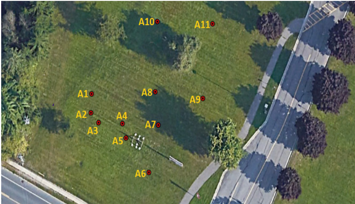
Figure 11: Anomalies in the South West Section, mapped by Ground Scan Ltd.
