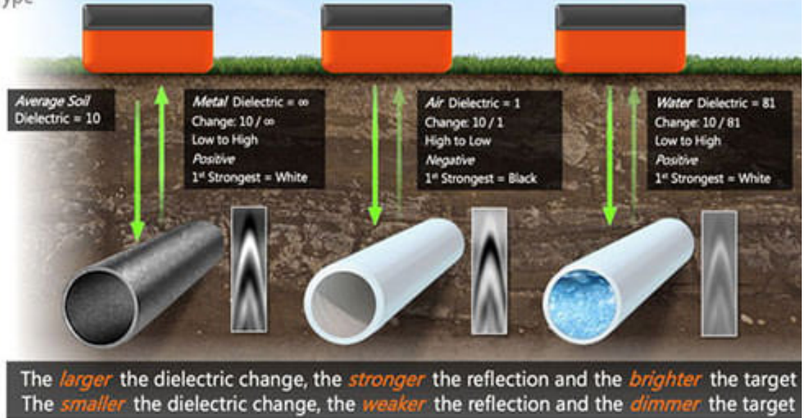
Figure 3: Image showing the different responses as expected from different building materials. Metal, PVC and water filled pipes all have distinctive responses allowing them to be identified using GPR. Image credit: Geophysical Survey Systems Inc. (2025).
