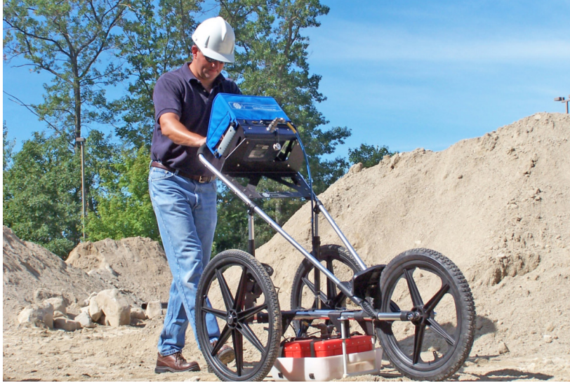
Figure 5: GPR Data Collection Cart Equipped with a SIR 3000 Data Collector.
